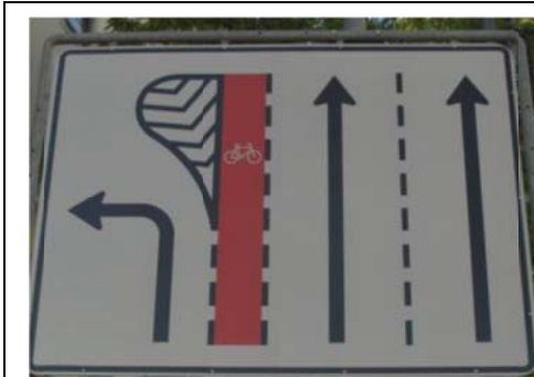
Cyclists return to carriageway ahead of left turn to a cycle lane offside of the turning lane. Only works for with-flow cycle facilities. (Phil Jones Associates)
