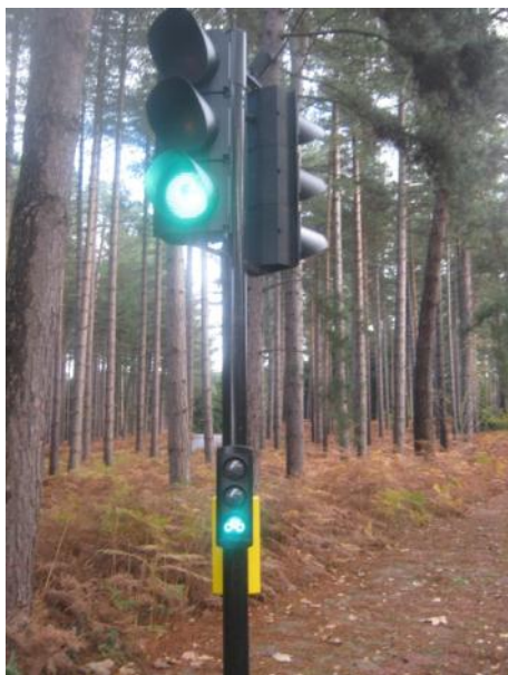
Example of low level signal aspect on trial at Transport Research Laboratory
