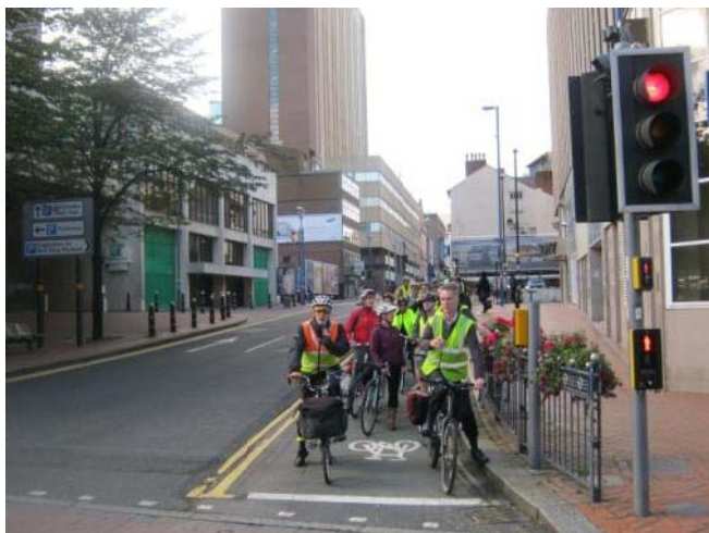
This separate signal phase enables cyclists on Hill St to cross over to a contraflow track in Hurst Street on the opposite side of Smallbrook Queensway.
