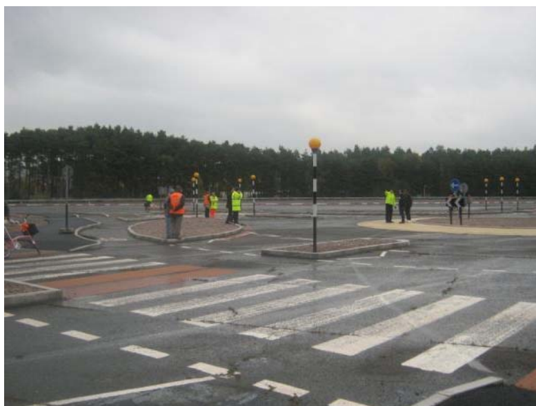
Dutch style roundabout trial at Transport Research Laboratory
