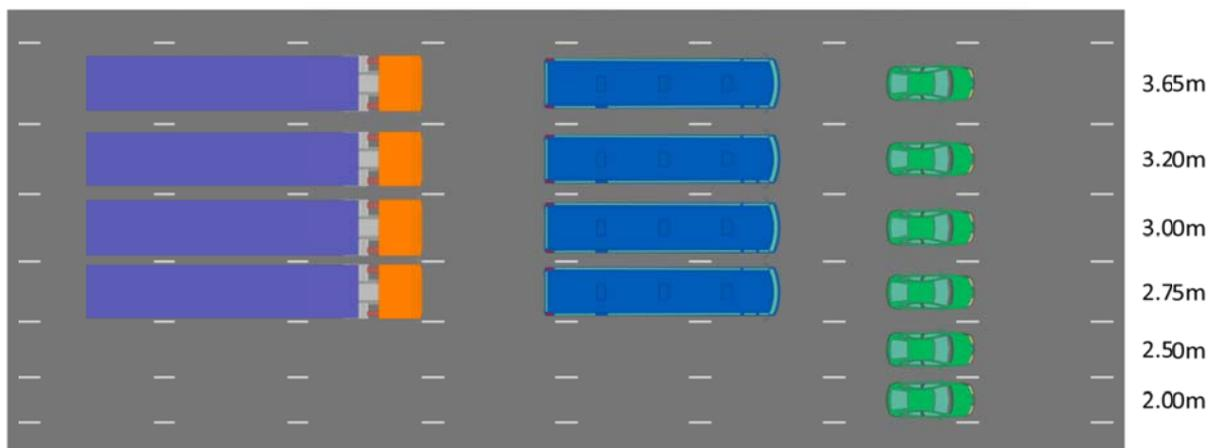
Figure 6 - Vehicles and Lane Widths<sup>5</sup>
