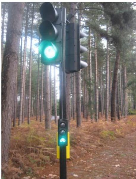
*Example of low level signal aspect on trial at Transport Research Laboratory*
