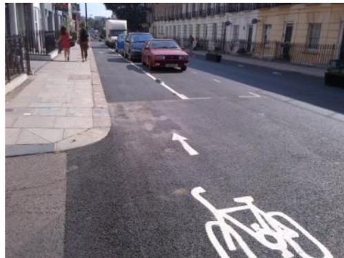
*Car parking can be used as a 'buffer' between the cycle facility and the live traffic as in the examples above. Ideally 0.5m gap should be left to protect cyclists from car doors. This arrangement is useful for contraflow facilities where cyclists are facing the drivers and so are at less risk from car doors.*
