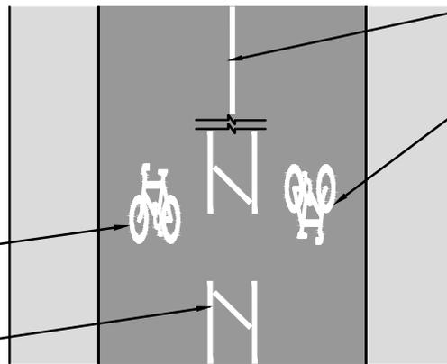
For carriageway widths <5.5m, carriageway centre marking to be omitted.
