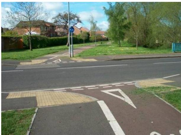
*Example of off-road cycle track along line of a footpath that crosses the footway of the road.*
