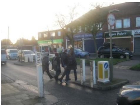
*Physical width restrictions (in association with a TRO restriction) can be used to exclude larger vehicles from using residential areas with narrow roads as through routes. Access for emergency vehicles (such as the gate in this photograph) must be retained.*
