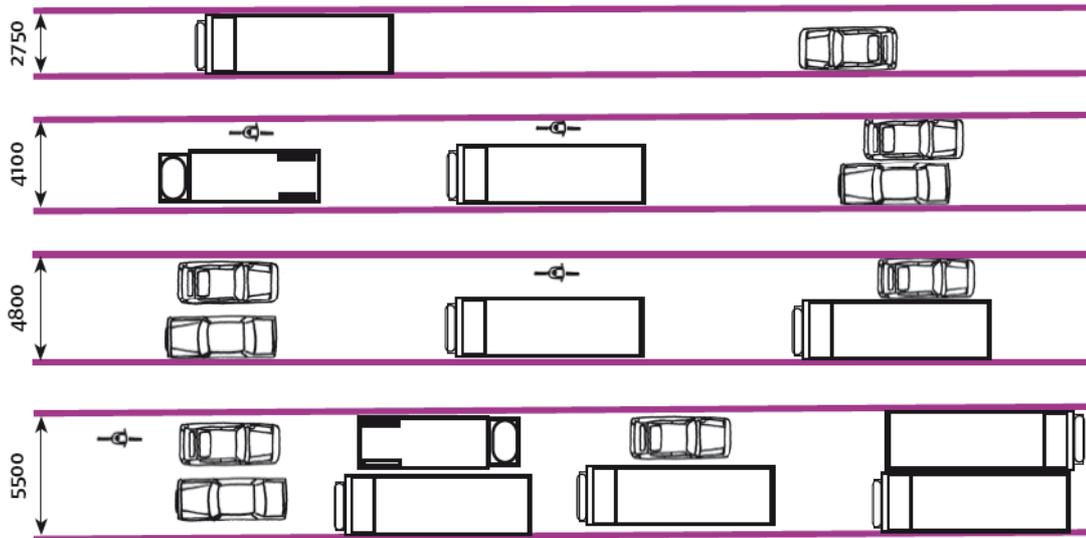
Figure 5 - Illustration of what various carriageway widths can accommodate<sup>4</sup>
