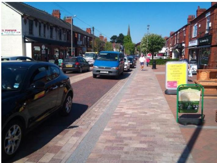
*Poynton: Removal of street clutter, use of textured central margin and side bars to visually narrow carriageway while still providing adequate width for HGVs. Cyclists use the all-purpose carriageway but can enter the footway at-grade to stop at shops etc.*
