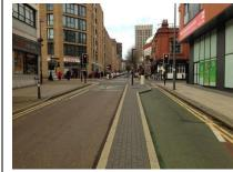
A contraflow is a cycle lane which runs in the opposite direction to the main traffic flow. This allows cyclists to use one-way streets in both directions, for example.
