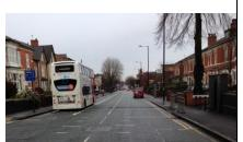
Dedicated lane for bus use, separated from the main carriageway with a solid white line. Cyclists can use bus lanes where a bicycle is shown on the blue bus lane signs.
