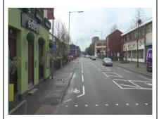
Advisory cycle lanes are identified by a broken white line. Vehicles may enter the lane when required. For example, advisory cycle lanes might be used to allow: buses to access bus stops; loading and unloading; and to be crossed in emergencies. Cycle lanes are identified using road markings and/or physical features.
