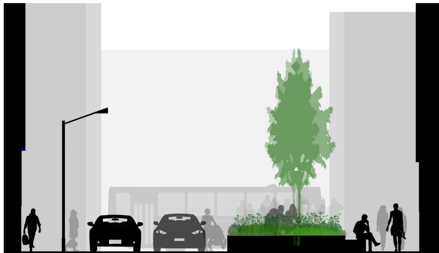
Pedestrian clear zone Carriageway City Greening Pedestrian clear zone
