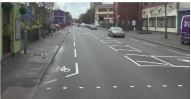
**Contraflow cycle lane -** is a cycle lane which runs in the opposite direction to the main traffic flow. This allows cyclists to use one-way streets in both directions.
