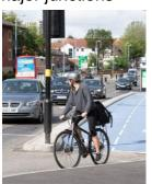
**Shared use footway/ cycle track -** pavements that are designed for both pedestrians and cyclists to use - identified with blue shared use signs and possibly with surface markings. Pedestrians and cyclists may share the space without separation or may be separated by painted white lines
