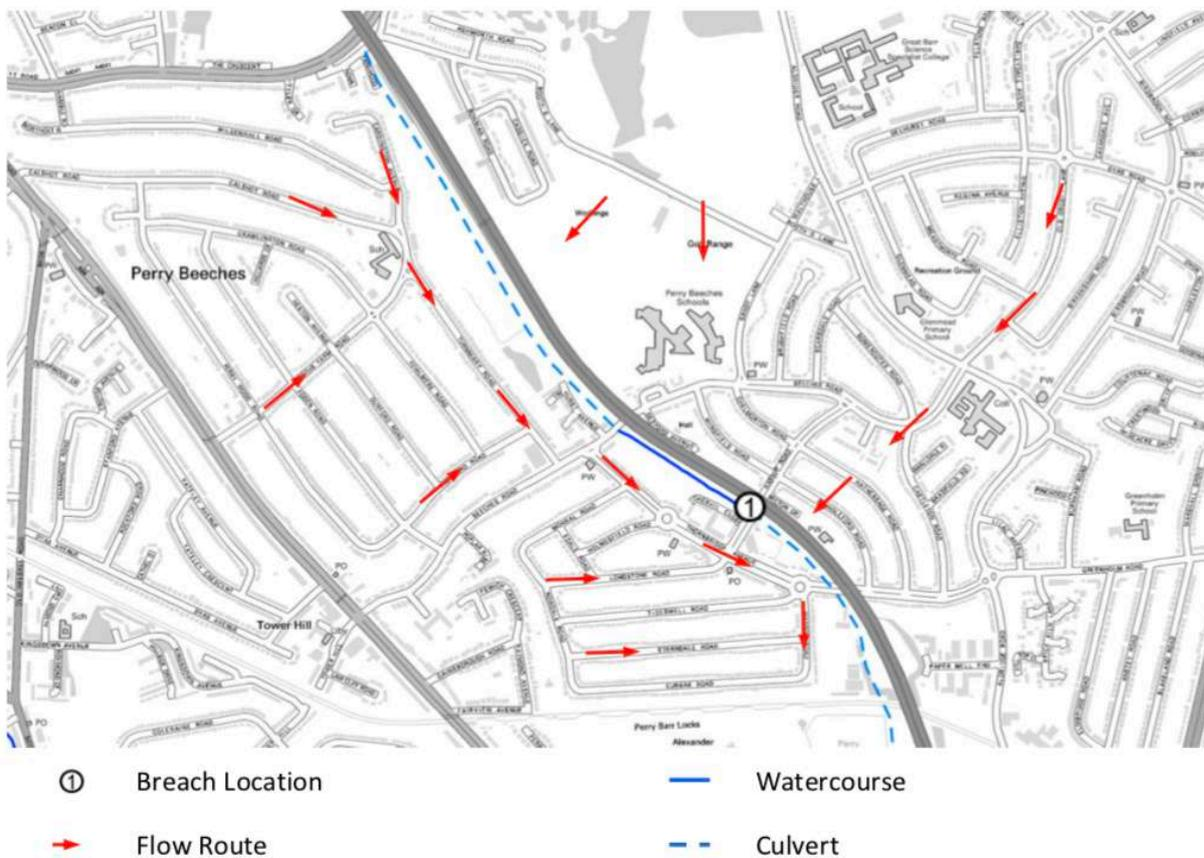
Figure 4-24 Potential watercourse breaches and flow routes
