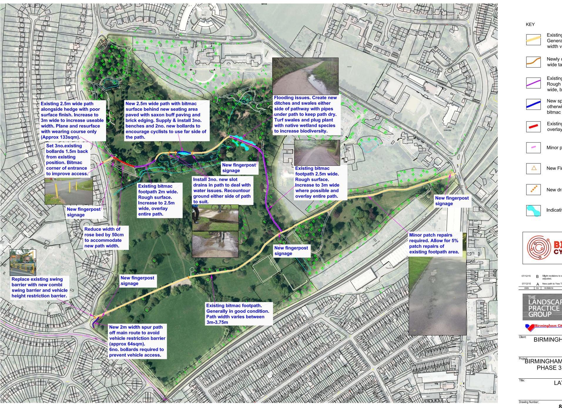
Existing bitmac footpath. Generally in good condition. Path width varies between 3m-3.75m
